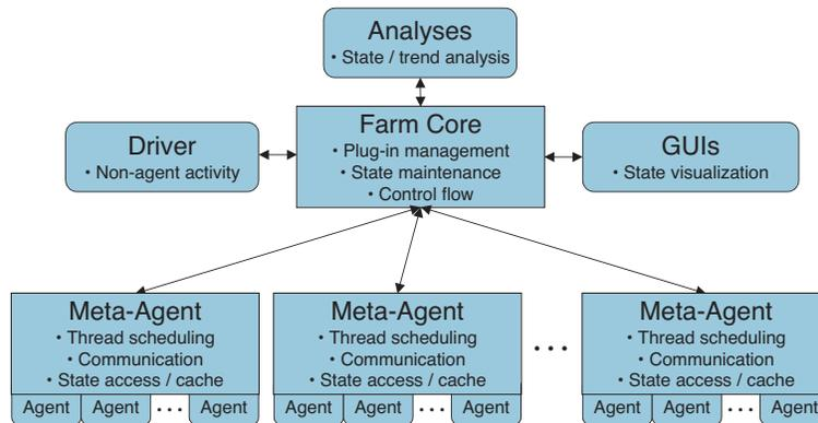
Fig. 2. An example of Farm's component architecture.
